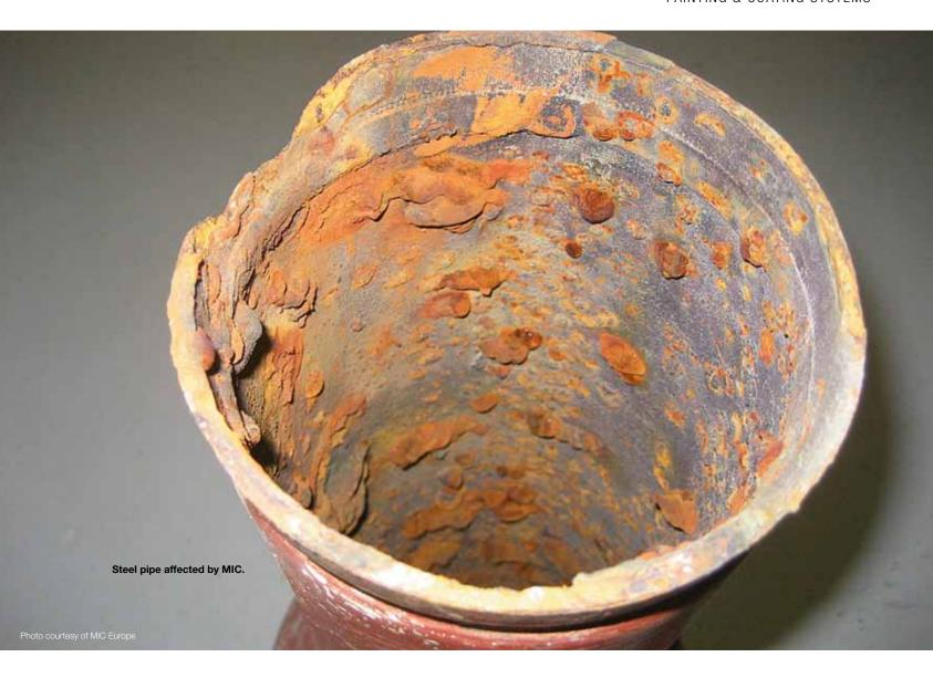
crop up in still water, particularly when the temperature starts to rise. Fire system mains constructed of stainless steel AISI316, which are filled with still water, have been found to leak within a year.
